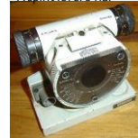
Mechanical spirit level clinometer with micrometer adjustment
